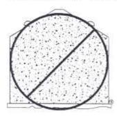
Grain piled in the roof area must not block the roof vents. Blockage of the roof vents with grain will restrict the effective vent area by 95-98%. Therefore, if grain is allowed to block roof vents, the vent area is virtually eliminated. The area above the surface of the grain must allow free movement of the air to the vents.
