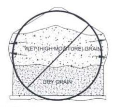
Because of the possibility for excessive hoop stresses caused by grain kernels expansion, it is recommended that grain bins be managed to prevent grain moisture contents from increasing more than 2% during storage. In addition, it is not advisable to have grain moisture content variations more than 5% in a storage bin.
