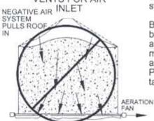
Maximum recommended pressure differential in the roof area is 1" static pressure.
